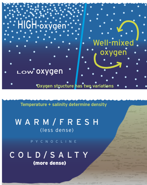
Figure 3-6 Stratification and oxygen structure in estuarine waters.
